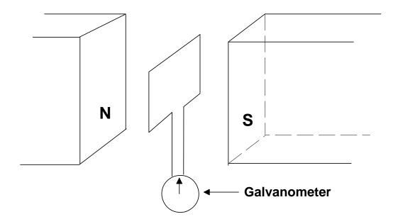
It was noticed that as the loop was moved a current flowed momentarily in the loop detected by the sensitive, centre zero galvanometer.
